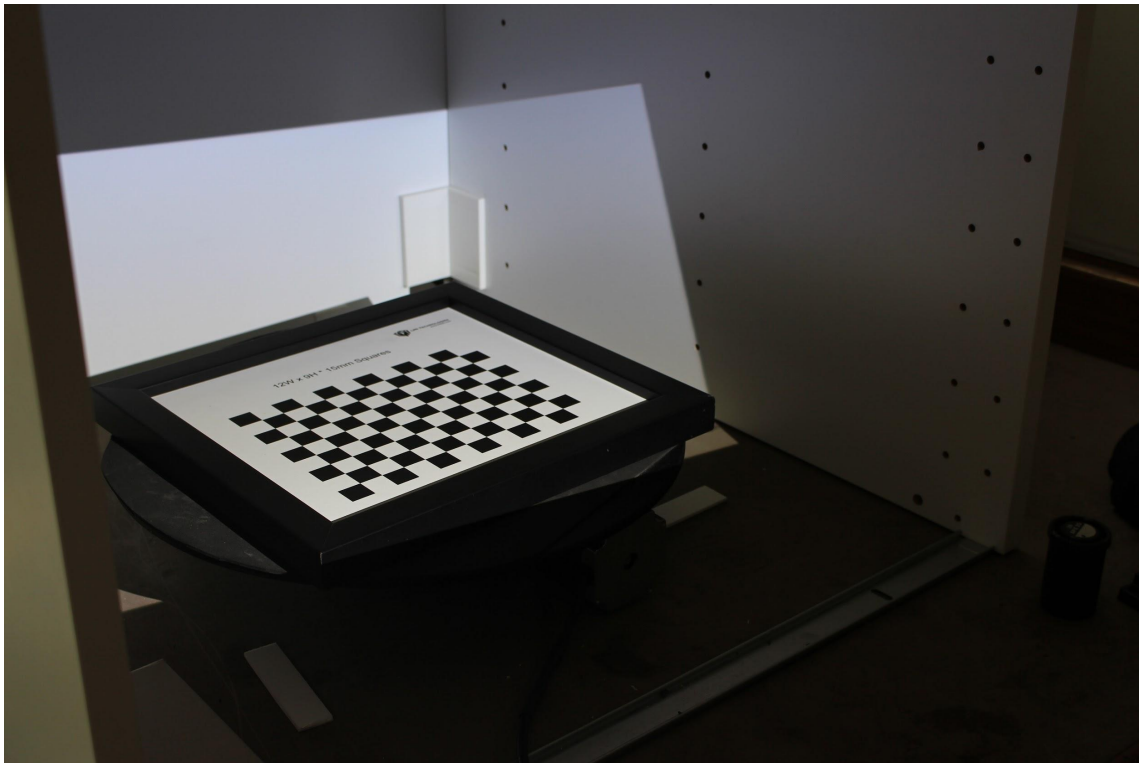
Figure X: Calibration plate lying flat on the turntable in order to calibrate the turntable.
