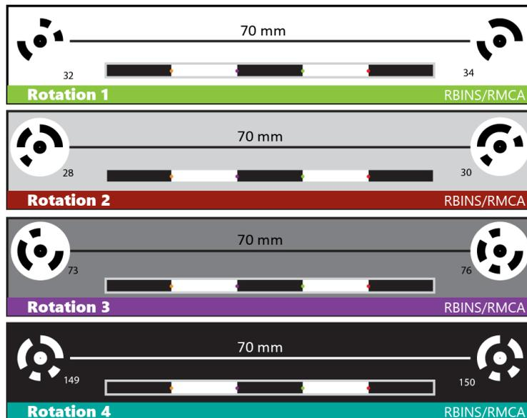
*Example of scales with photogrammetry targets*
