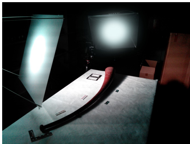
Figure 2: Multispectral photogrammetry setup used to digitize the horn.
